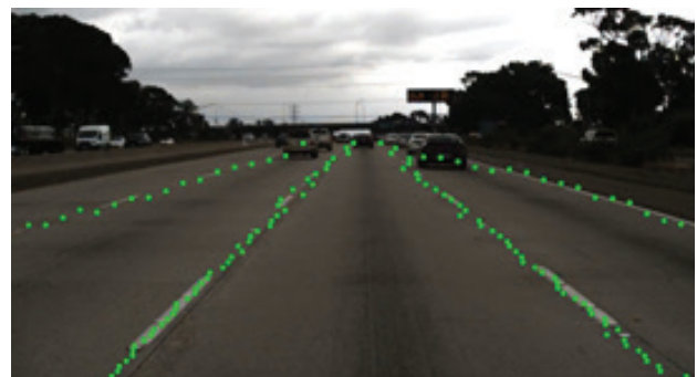
Fig. 8 Lane detection result for UFLD-HAOC (ResNet_34)
