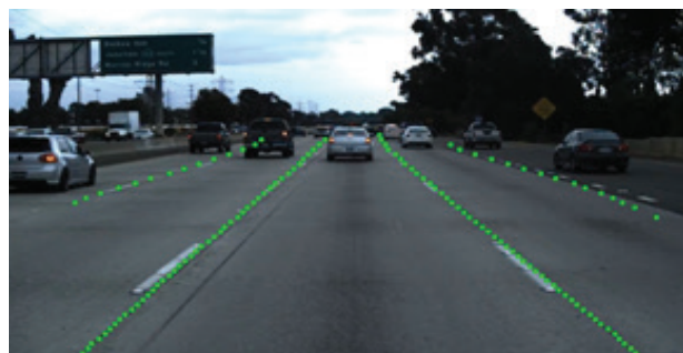
Fig. 7 Lane detection result for UFLD-HAOC (ResNet_18)
